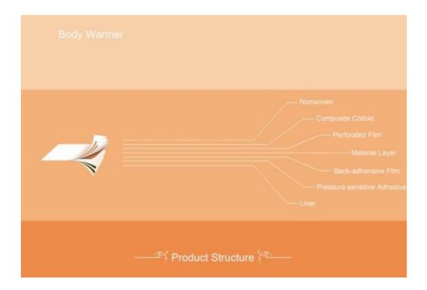
Body Warmer use the theory of Primary Battery to accelerate the Oxidation reaction. when the iron powder meet the O2, the product will start heating.
